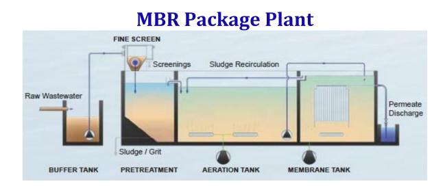
A membrane bioreactor (MBR) is a wastewater treatment process combining membrane filtration with biological treatment. This innovative technology offers several advantages over the conventionally activated sludge process. Among these advantages are higher biomass concentration, elimination of the settling unit and improved effluent quality.
